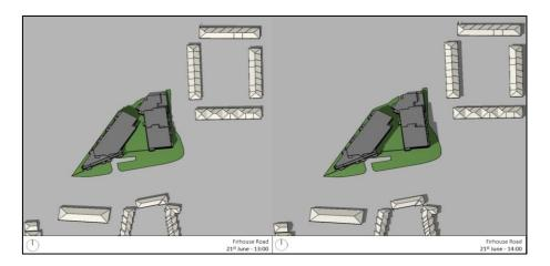
Figure 39: Overshadowing Images on June 21<sup>st</sup> at 1 p.m. and 2 p.m.
