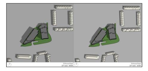
Figure 37: Overshadowing Images on June 21<sup>st</sup> at 9 a.m. and 10 a.m.
