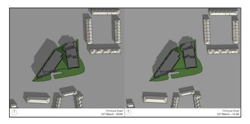
Figure 33: Overshadowing Images on March 21<sup>st</sup> at 10 a.m. and 11 a.m.
