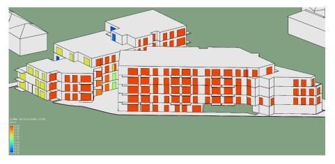
Figure 25: Sunlight Exposure March 21<sup>st</sup> (EN 17037 Min Recommendation) – North West Elevation
