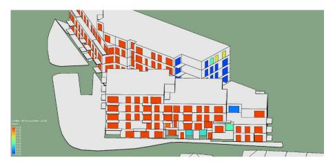
Figure 24: Sunlight Exposure March 21st (EN 17037 Min Recommendation) – East Elevation
