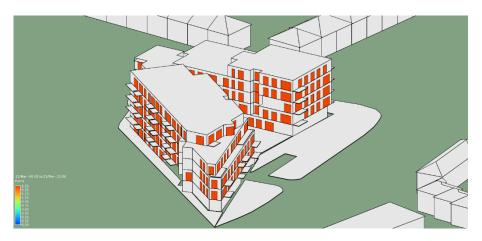
Figure 26: Sunlight Exposure March 21<sup>st</sup> (EN 17037 Min Recommendation) – South West Elevation
