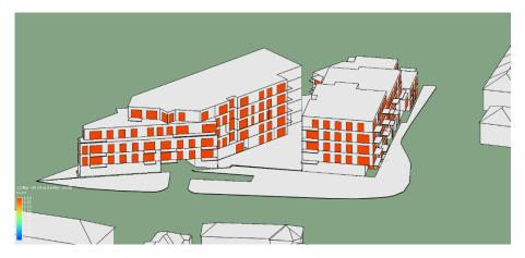
Figure 23: Sunlight Exposure March 21<sup>st</sup> (EN 17037 Min Recommendation) – South Elevation
