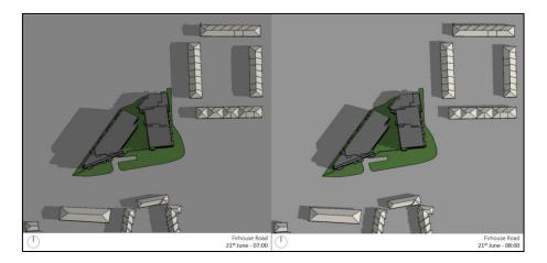
Figure 36: Overshadowing Images on June 21<sup>st</sup> at 7 a.m. and 8 a.m.
